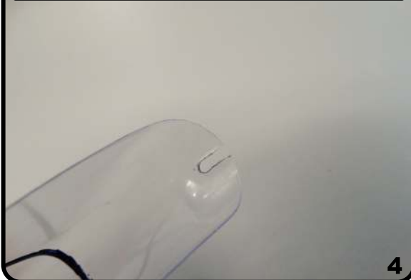
Cut an open slot at the front of the canopy
