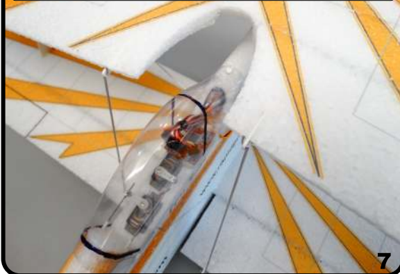
Final canopy and gear installation
