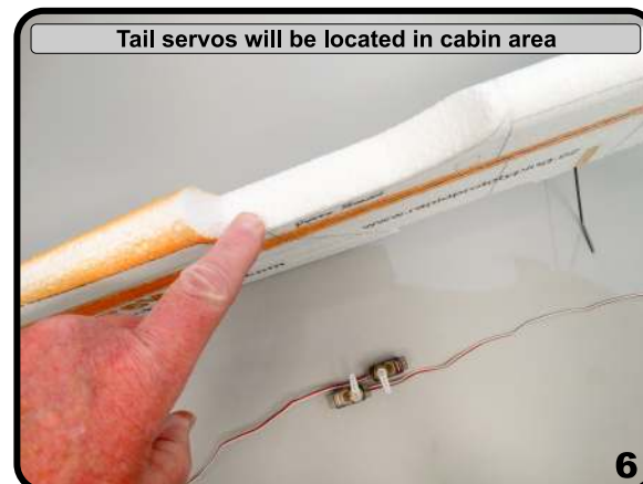
Arms can not extend beyond the side of fuselage
