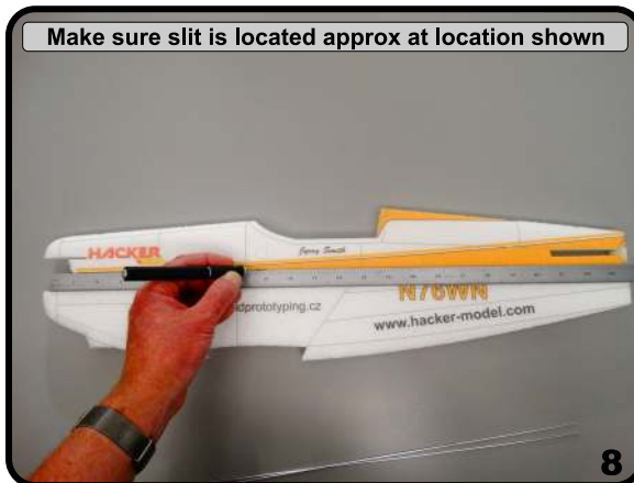
Press rod in flush and CA. Repeat for other side
