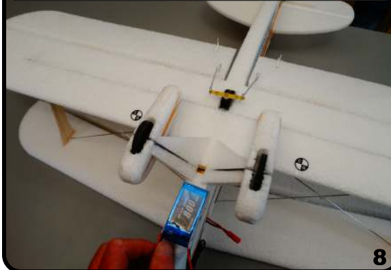
Double check battery location for CG
