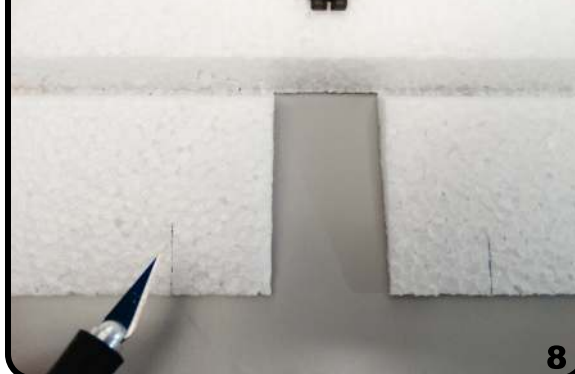
Make a mark and cut a slot all the way thru...
