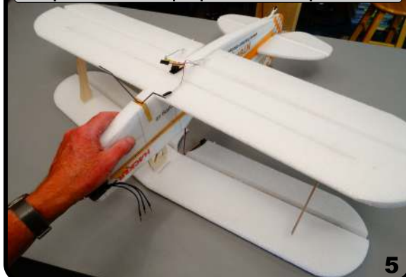
Flip over and line up tops slots with top of struts
