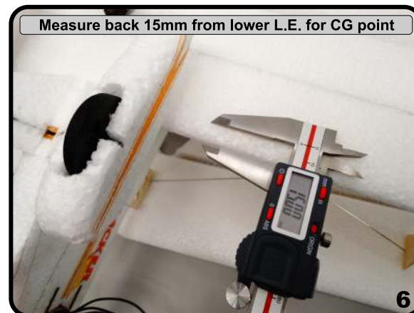
Locate the ESC as required for proper CG
