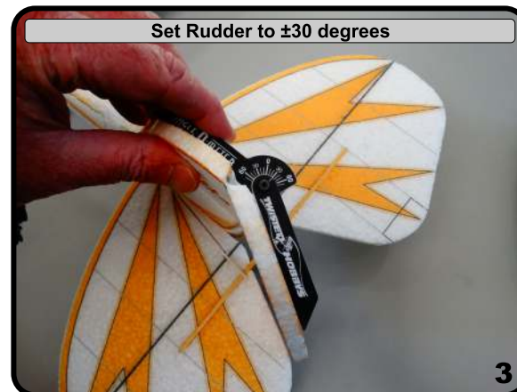
Close-Up of Rudder push rod and plastic guide
