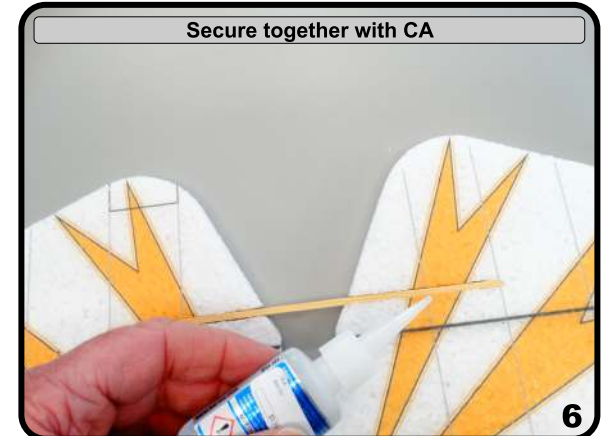
Slide in the elevator with top side facing up
