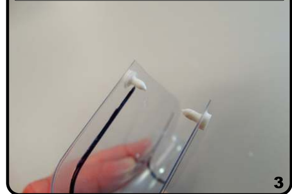
Locate white canopy pins and secure with Med. CA
