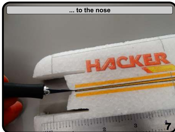
Make sure slit is located approx at location shown
