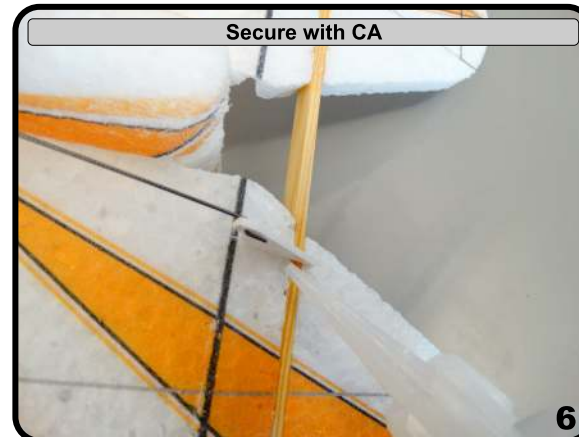
Hold in position with stick pins
