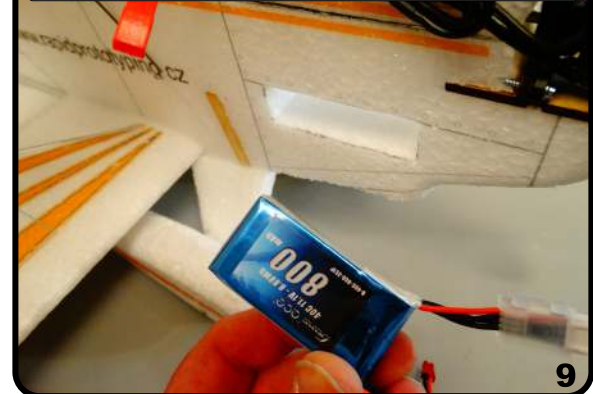
Cut a hole for snug fit of your battery
