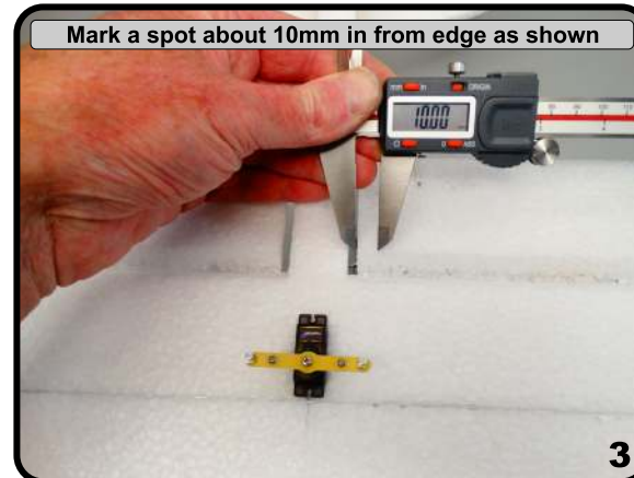
Insert the horn with hole over hinge line
