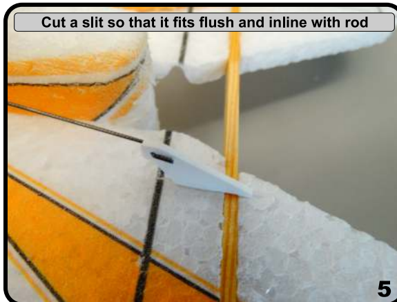
Test fit - make sure all surface match up flush
