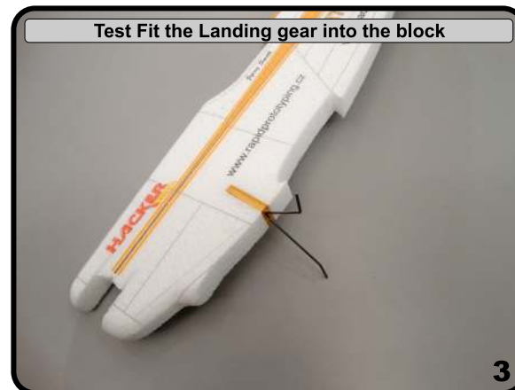
Cut a slit about 3mm deep from the tail...
