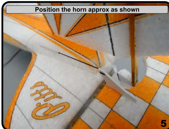
Center servo and surfaces and clip extra wire
