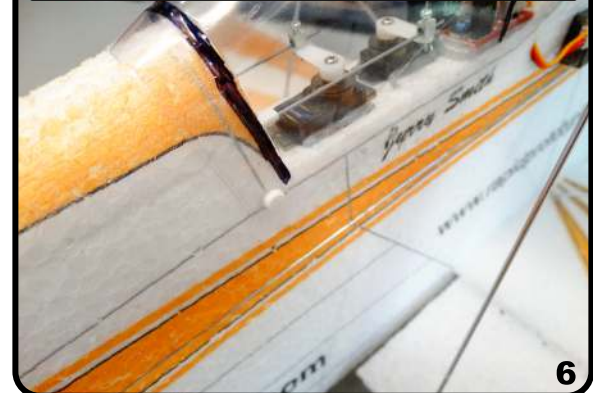
Poke the rear pins into the foam (do not glue)
