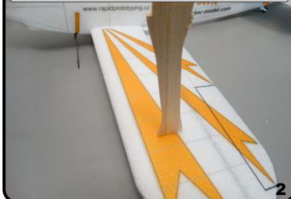
Locate outer strut slot
