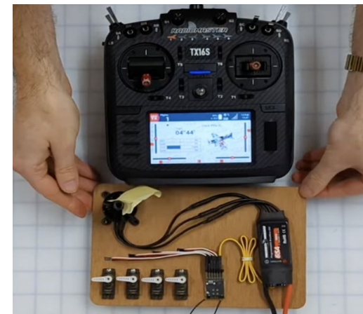
Hook up the entire electronic system as shown. Mount and center the control horns and servos Test for proper operation of all items
