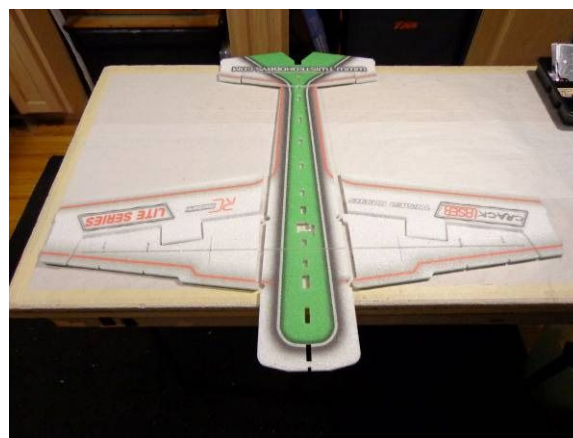
Locate the items shown above and apply a tack coat to the mating surfaces and let sit for approx 5 minutes before joining together
