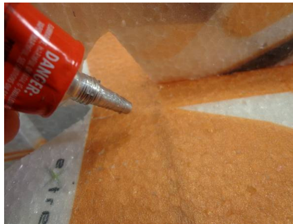
When happy with the fit, remove the horn and squeeze some glue into the slit, re-install the horn, check alignment and wipe away any extra glue
