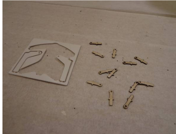
Next up is the control horns for the tail and the control rod guides
