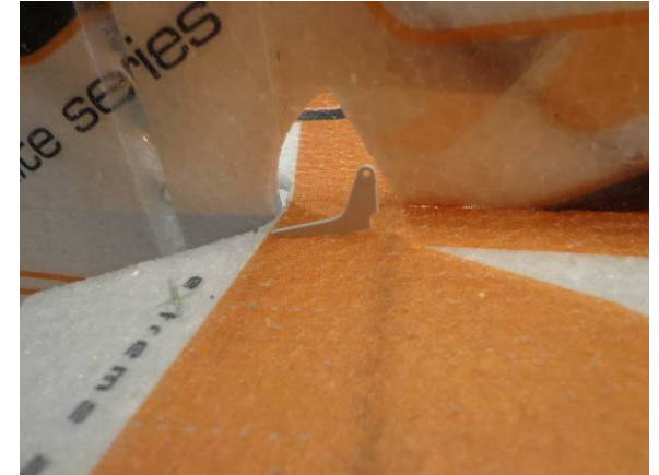
Test fit the horn into the slot, it may need to be cut thru with a hobby knife. Hole in the horn should be directly above the hinge line. Picture shows the horn but not full seated yet
