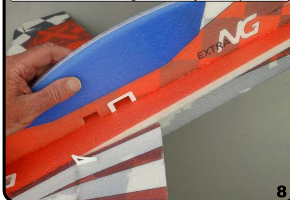
Left side of the fuselage - RUD tray in rear position
