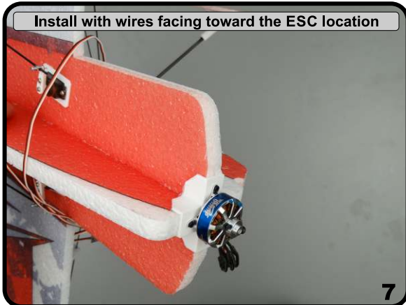
With FoamTac locate RX - ESC - and route the wires
