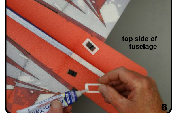
Attach the trays with FoamTac - Center on cutouts
