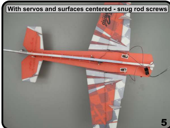
With FoamTac locate RX - ESC - and route the wires
