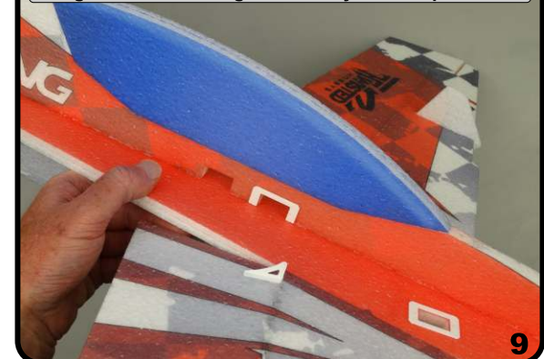
Right side of fuselage - ELE tray in front position
