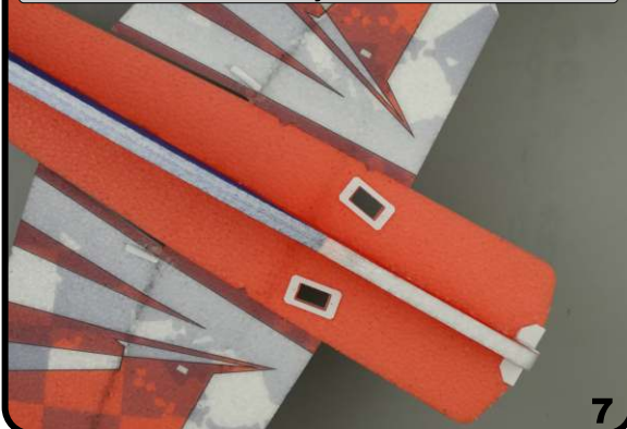
Aileron trays installed
