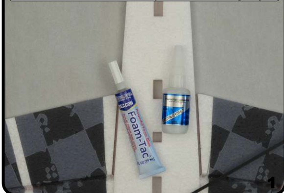
Use FoamTac for Durability / Use CA for Rigidity
