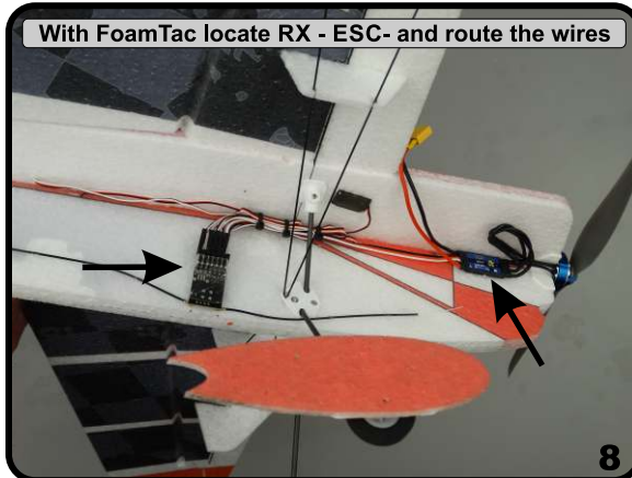
Install with wires facing toward the ESC location
