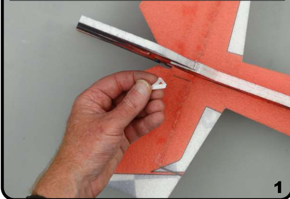
Elevator horn - install like was done on the ailerons
