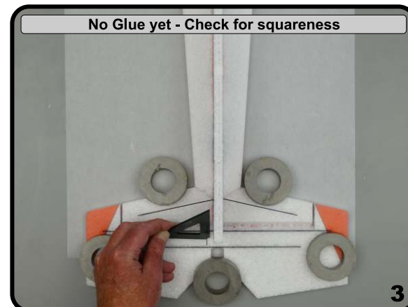
Note that there is a "V" on the fuselage and block...
