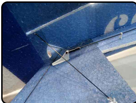
Center the servo, center the elevator. Slide the rod thru the guides from the front of the air craft. Trim the rod and attach the clevis as was done with the rudder.
