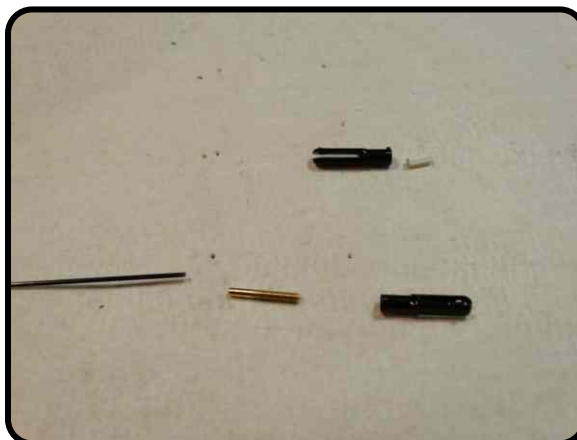
Build the elevator control rod in the exact same manner as was done with the rudder control rod. Note - don't install the clevis with the white tube just yet.
