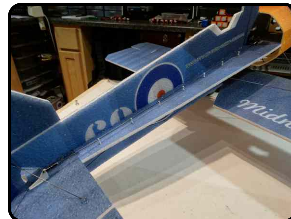
Picture of completed control rod assembly.
