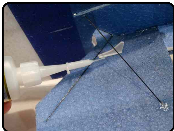
... and secure with thin CA and Kicker.
