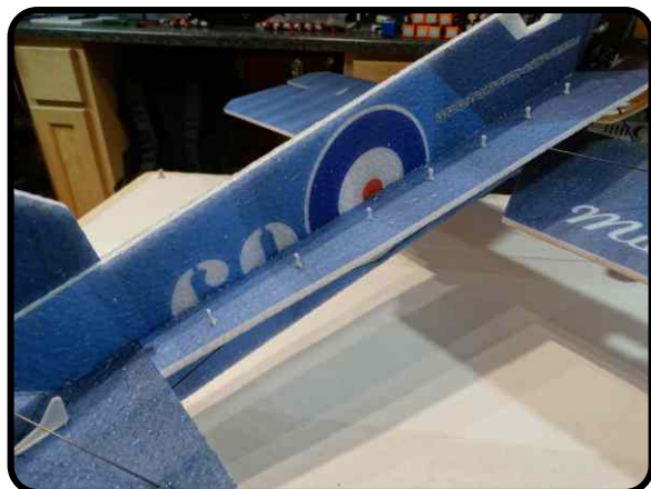
Install them into the precut slots, line them up and secure with CA and Kicker.
