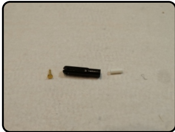
Locate another one of the black clevis parts, one of the small white tubes and the mating brass pins
