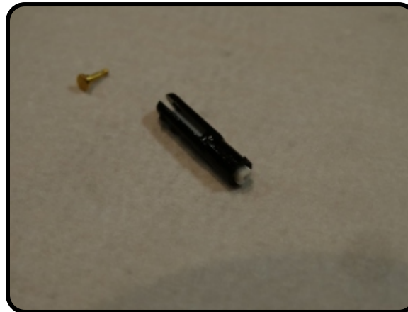
Install the white tube into the end of the clevis as shown. It will be a tight fit.
