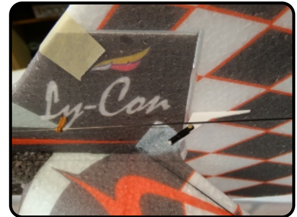
Attach the clevis from the previous step to the rudder control horn.
