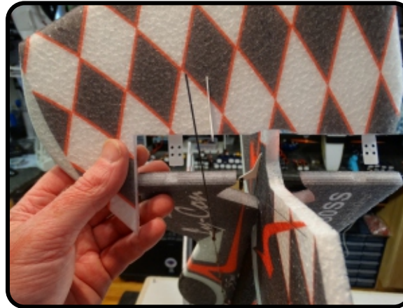
Make matching slits in the stab on the fuselage and press the rudder/hinge assembly into them.
