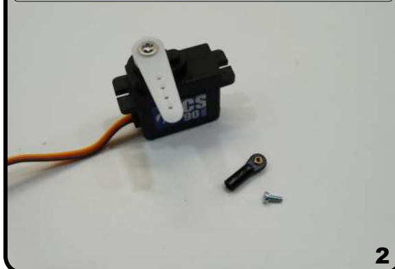
Locate rudder servo and ball link
