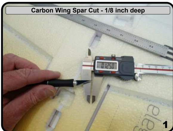
Cut 1/8 inch deep from wing tip to wing tip
