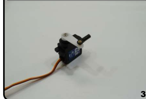
Attach ball link as shown. Use thread locker
