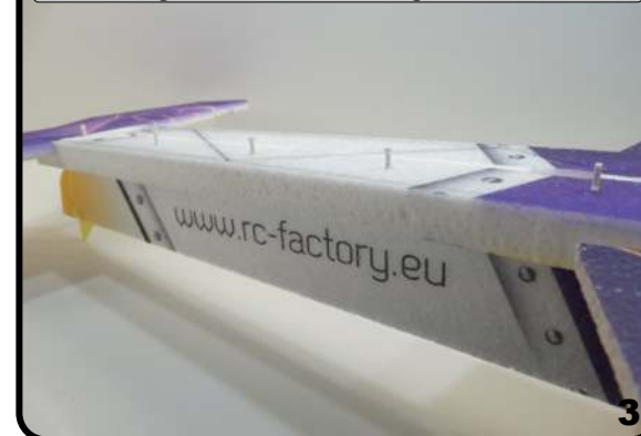
Place guides into holes - No glue at this time
