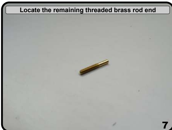
Thread it onto ball link attached to the rudder servo
