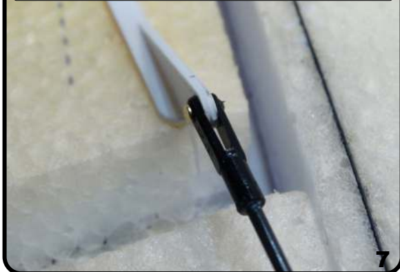
Squeeze flush and make sure pin is fully seated
