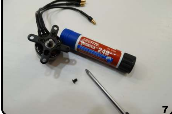
Mount the back plate with thread locker
