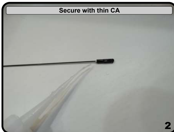
Thread rod piece with clevis thru guides from rear
