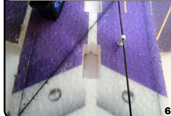
... cut out clearance for the wires
