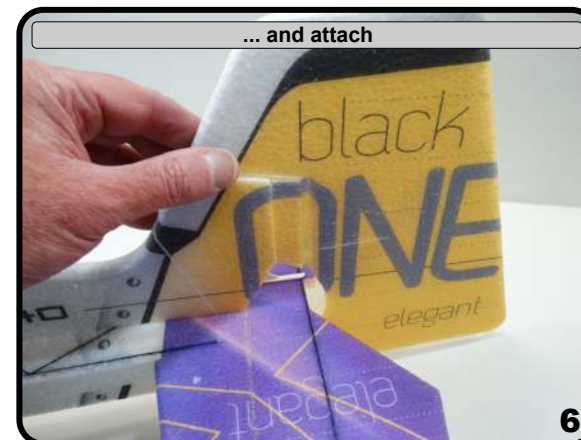
Locate the rudder control horn
