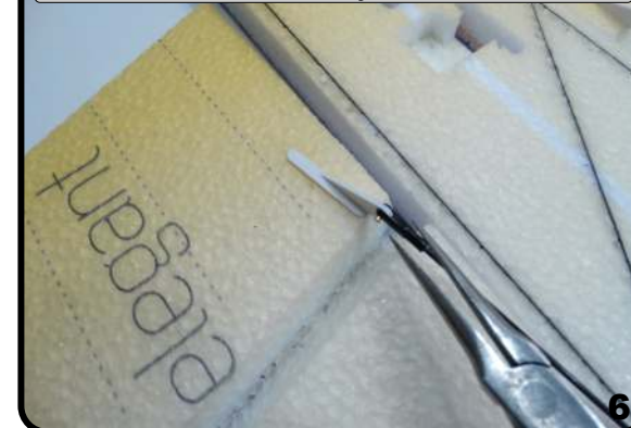
Attach the rod & link assy to the control horn
