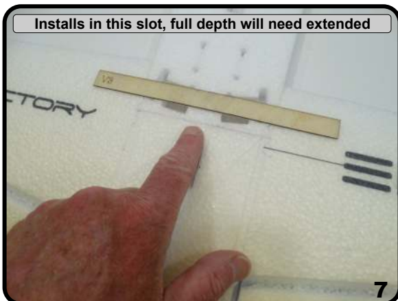
Make the extension cuts all the way thru the wing
