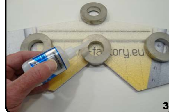
Constrain the assembly flat and secure with CA
