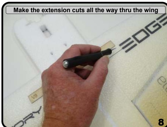
Installs in this slot, full depth will need extended
