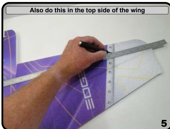
Make the extension cuts all the way thru the wing
