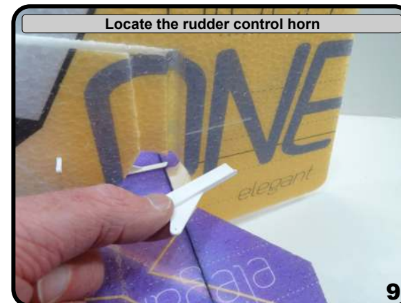
Break them apart and stick into holes - no glue
