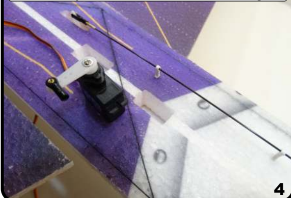
Electronically center the servo and arm at 90 degrees
