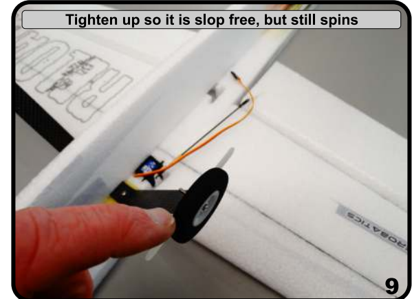
screw>wheel>nut>washer>strap>LG>washer>nut
