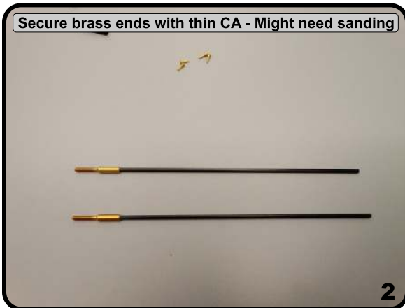
Repeat for other control rod & secure with thin CA
