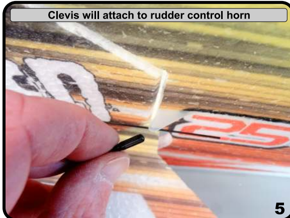
Slide rod into back of clevis and spacer
