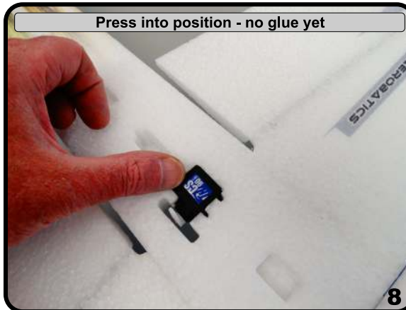
Fit into the pocket and cut slits for mounting tabs
