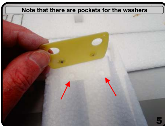
Set into place - make sure it's square to fuselage
