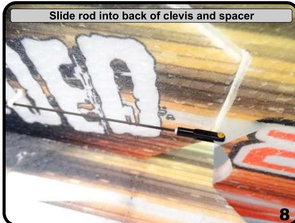
Center Servo and Rudder - Cut rod where shown
