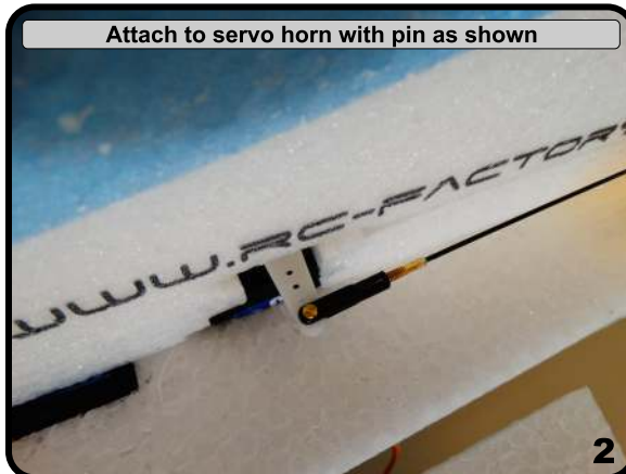
Clevis will attach to rudder control horn
