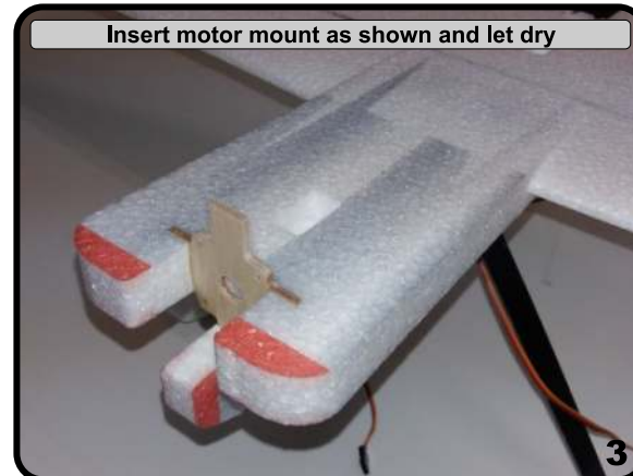
Cut a slit and install as shown - No glue yet
