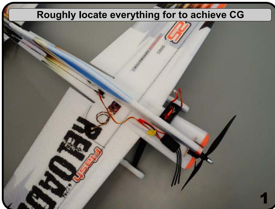
Bottom view showing component locations
