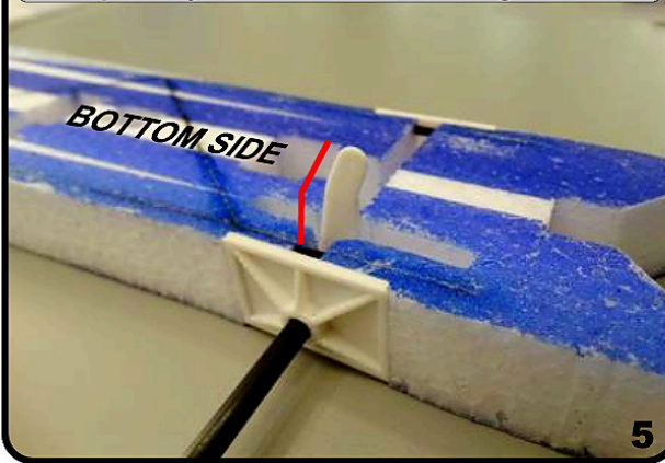
Push part way in then install horn noting orientation
