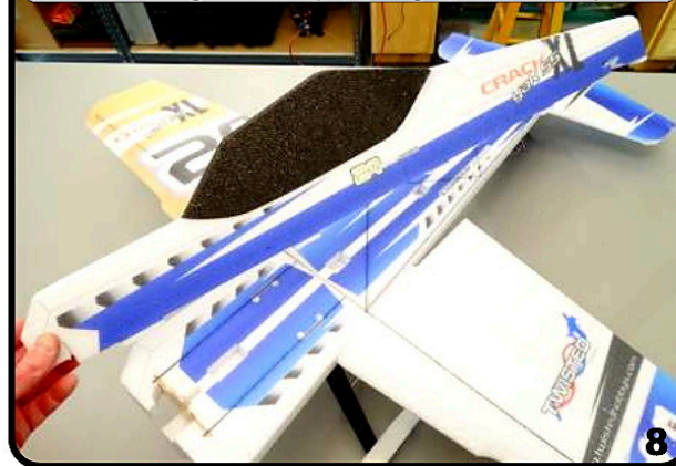
Test fit and glue the top fuselage on - make square
