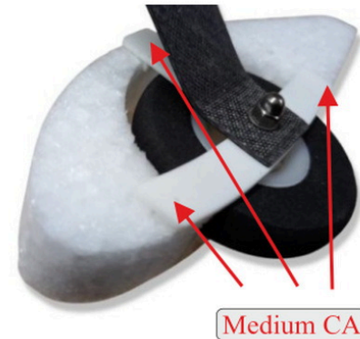
Apply Medium CA at all contact points
