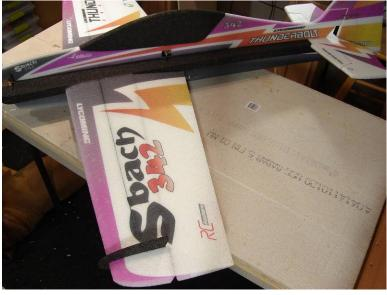
Lay down a thin bead of Welders on the top and bottom of the wing along the reference line, and on the inside of the SFG, spread smooth and allow to tack up. Once tacked up spread the SFG and carefully position it parallel to the line you made a press together to create the glue joint.
