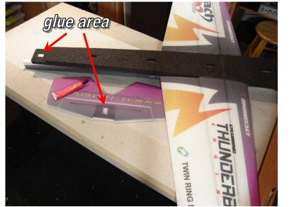
Apply Welders to the contact areas, spread smooth and allow to tack up.
