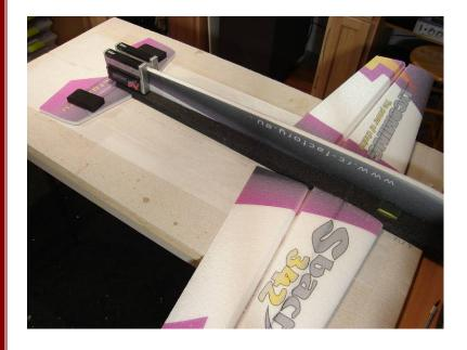
Carefully attach the Elevator so that it is square and true, apply a little weight and allow the glue a little time to fully set up.
