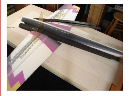
Once the glue on flat surfaces has tacked up, apply Welders to the sides of the tabs and assembly. Check for squareness and tweek from side to side if necessary.
