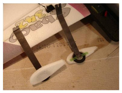
Locate and glue the Wheel Pants to the Wheel pan tabs. The included 2.9x6mm wood screws are used to attach the strut assemblies to the Fuselage. Landing Gear can be installed or removed easily by simply loosening and/or tightening. MAKE SURE WHEN GLUING ON THE WHEEL PANTS THAT YOU MAKE A LEFT AND RIGHT ASSEMBLY.
