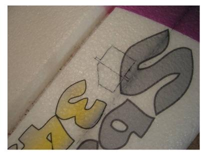
Mark and remove the necessary foam needed to mount the servo. Make the recess slightly smaller than the Servo so that it is a snug fit, but is still allowed to sit flush. Standing the servo up is an option if wanted.
