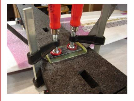
It is important for this assembly to have a minimal amount of slop. In order to get the proper depth of the Strirrups, use the LG and some clamps to hold everything accurately in place while the glue dries. The LG needs to be removeble, so make sure that there is no glue that squishes out and creates a bond to the LG Plate or Stirrups. Do not over tighten the clamps.
