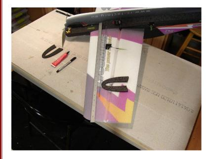
If needed scape away any glue that might have gotten on the pivot point areas of the hinge pieces. Use a small needle nose plier and little screw driver for assembly. Do not over tighten the scews, the Rudder should move freely back and forth without binding or excess slop. Put a small dab of Welders on the Nut once the everything is set.
