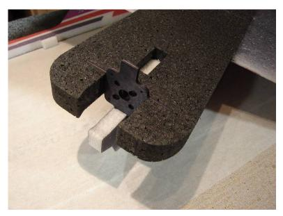
Glue the Firewall to the lower assembly as shown, make sure to glue in all areas of contact.
