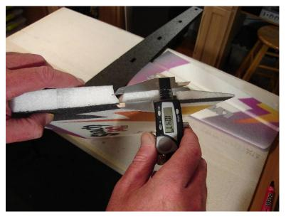
Make a reference mark as shown at the center of the inside root of the wing. This in conjunction with the tip of the leading edge will be used to line up with the carbon strip in the fuselage backbone to aid in aligning the two pieces for 0 degrees of incidence.
