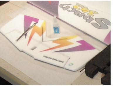
Flip the Elevator over to the top side and install the 1x3x100 strips as above, into their respective pre-cut slots.
