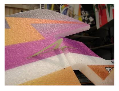
Move the Rudder back and forth to approx 45 degrees and note how much clearance is needed between the rudder and the fuselage, make a small mark on the hinge pieces, so that once this is dis-assembled for gluing purposes you can accurately re-locate the hinge pieces.
