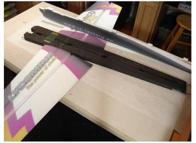
Apply a thin layer of Welders to the contact areas of both pieces, and smooth to a thin layer and allow to tack up. Do not put any glue on the sides of the tabs at this time, as those areas will need to "slide" together, glue will be added to this area just before assembling the lower Fuselage to the Backbone.
