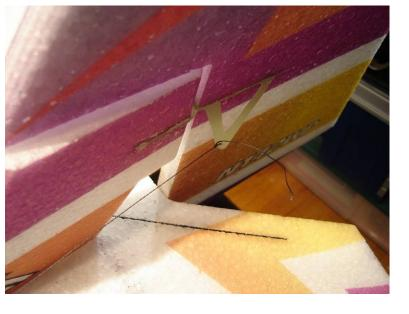
Attach the Kevlar cable to the Rudder control horn as shown, tie a knot and set with a dab of thin CA. Repeat for the other side of the horn.
