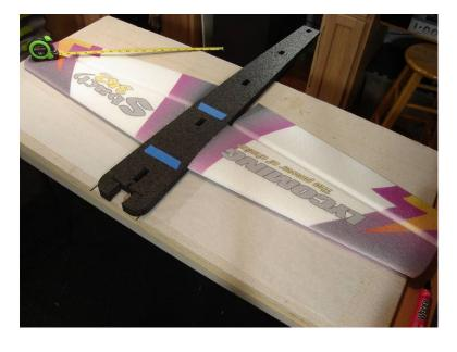
Mark with tape or a marker the area of the fuselage backbone that will come into contact with the wing roots. Also at this time check that when fully seated against each other that the wing halves are located symetrical in relationship to the fuselage backbone.
