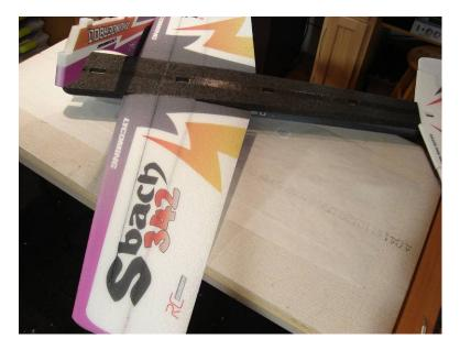
Apply a thin layer of Welders to the contact areas of both pieces, and smooth to a thin layer and allow to tack up. Do not put any glue on the sides of the tabs at this time, as those areas will need to "slide" together, glue will be added to this area just before assembling the upper Fuselage to the Backbone.
