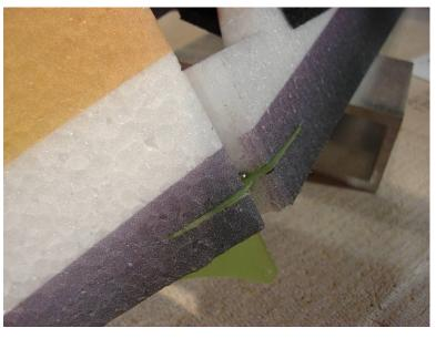
Locate the fuselage side of the rudder hinge (item 1- 2x), pin together with the M2 screws and cut matching slots in the fuselase. Care should be taken so that the rudder control surface lines up with the bottom of the fuselage and that there is some clearance between the rudder control surface counter balance and the top of the fix part of the rudder on the fuselage.
