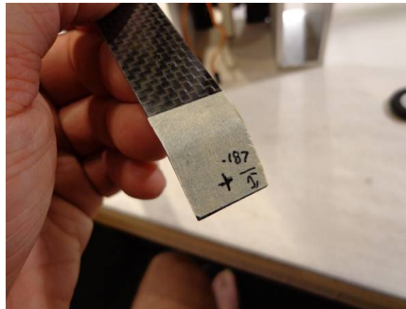
Drill a hole for the axle screw, approx 3/16" up from the end, and centered in the width
