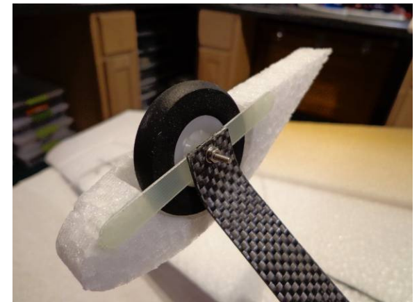
Attach the Wheel pant as shown, make sure the wheel has clearance to spin. Repeat for the other side.
