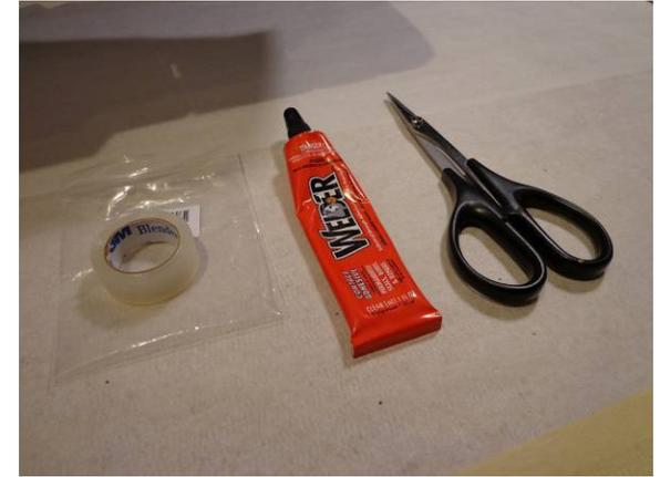
Apply little 1.50in long strips of blenderm to all the stressed areas of the airframe, starting with the legs of the motor mount...
