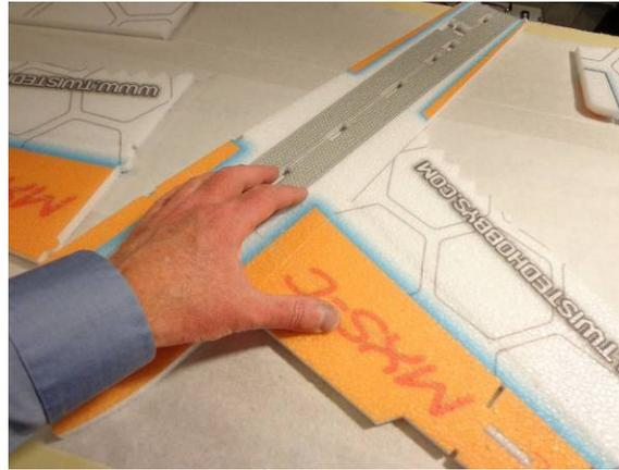
Once the glue has tacked up, carefully press wings back on for a permanent bond
