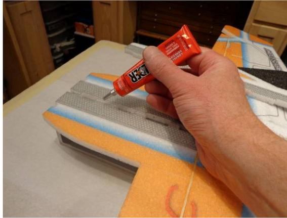
Glue the top fuselage on. Make sure to only apply glue to the flat section and the sides of the tabs during this step
