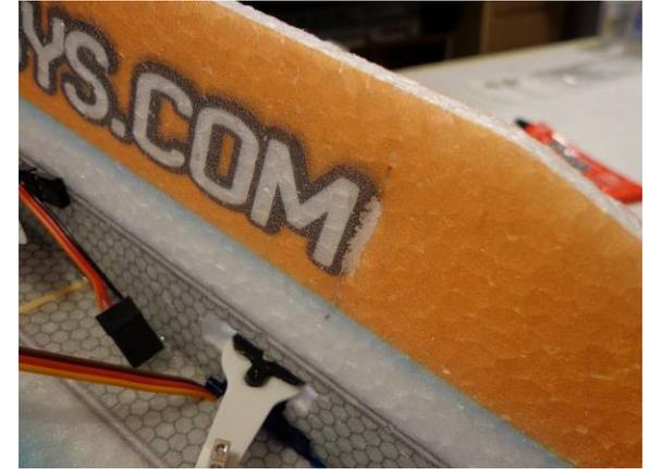
Apply Welders to the extreme ends of the cut out, where it captures the wood brace only. Leave the wider section in the middle free of glue for now.
