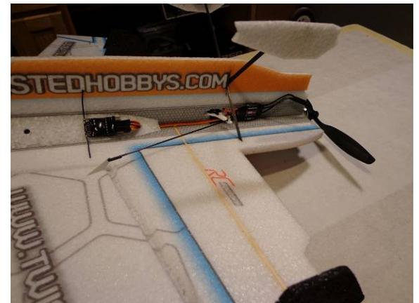
Mount the ESC as far back as possible. For rearward RX attach an extension long enough to the RX that allows the RX to reach the rear servos
