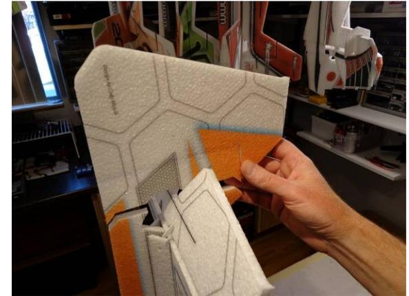
Glue the rudder on. Use the Tack up Method. Make sure it is in line and square with the vertical fuselage pieces
