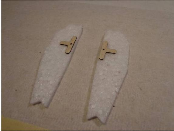
Glue the T-shaped wood pieces to the wheel pants. NOTE- be sure to make a LEFT and RIGHT hand version
