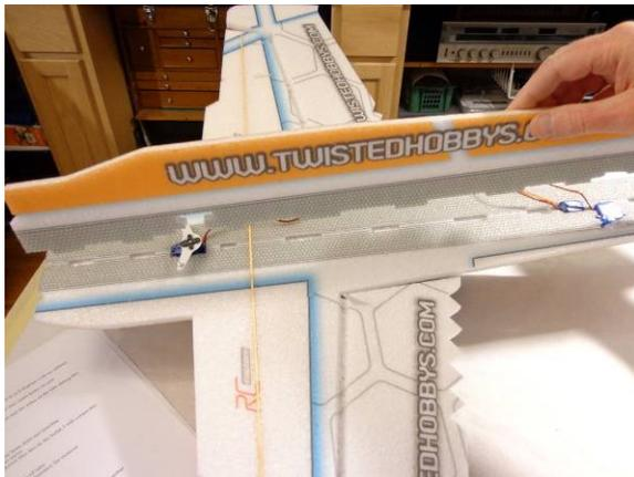
Install the lower fuselage. Use glue on full bottom surface and sides of tabs
