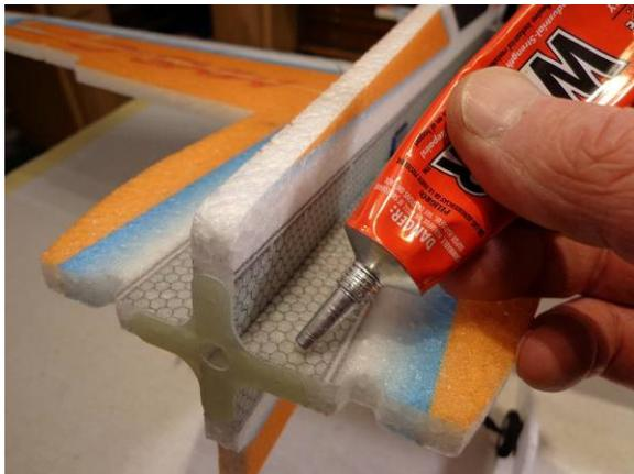
... first lay down a skim coat of Welders in all the area where the tape will be.
