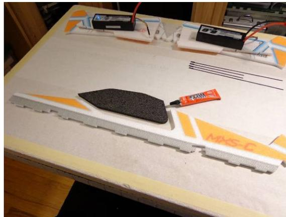
Also, as the hinges flex, glue the canopy. Put a bead of glue on the fuselage, press together and pull apart. Allow to tack up for five minutes
