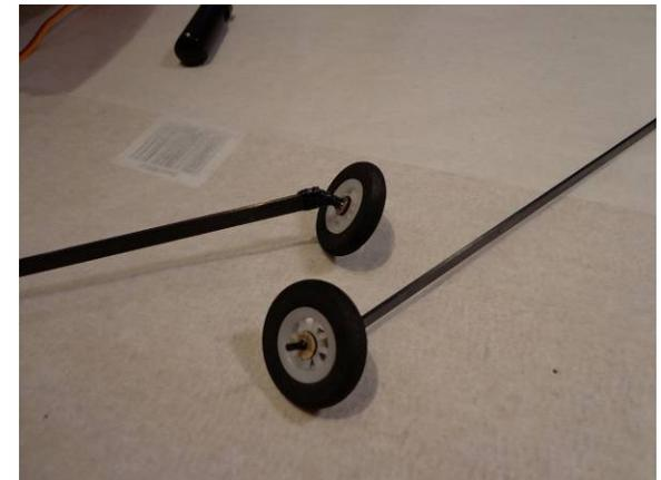
Drill the wheels out to fit the axles. Install and glue the inside washer then install the wheels. Install and glue the outside washer. Be Careful with the glue, wheels need to turn!
