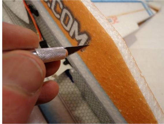
Next, install the landing gear onto fuselage, start by cutting out opening for legs and rectangular brace
