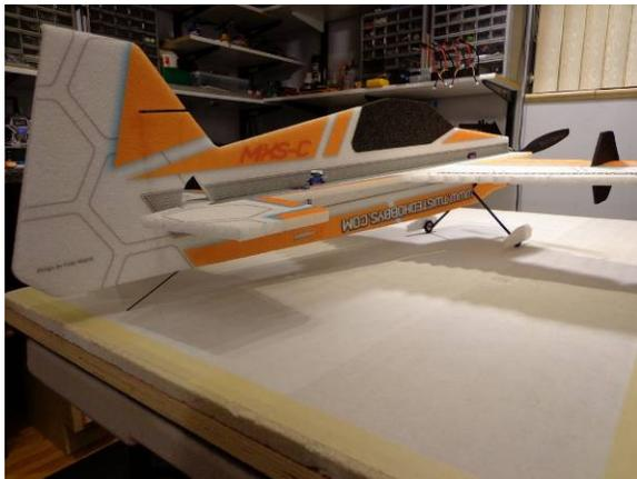
With the extra carbon rod from the Rudder, make a tail skid to protect the rear of the plane during ground operations
