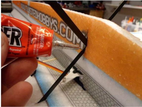
With the tip of the glue bottle, stuff some glue into the area where the struts cross thru the fuselage
