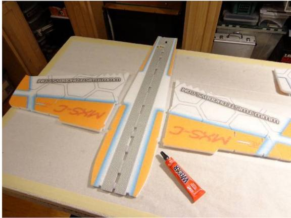
Remove the weights... Put a bead of glue on the wings where they meet the fuselage, press together, pull apart, let set for five minutes
