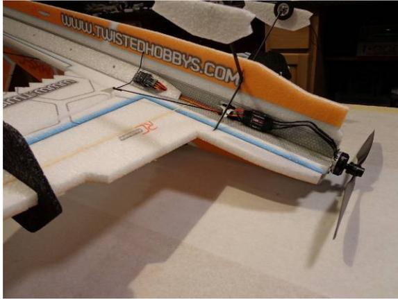
NOTE - This build was done with extensions on the rear servo side, ie Forward RX location. For Rearward RX location, the RX would be approx 1.0" behind the trailing edge of the aileron
