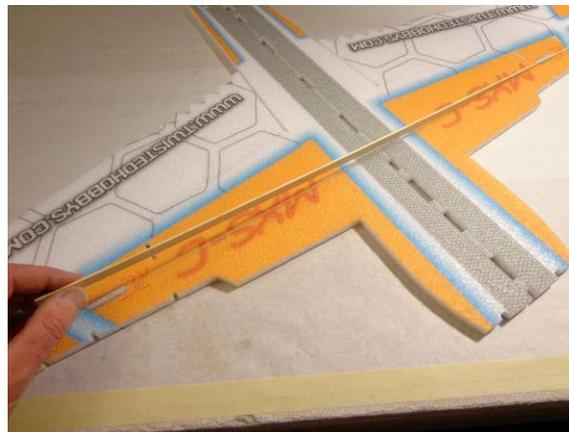
Test fit the spar, trim foam as needed
