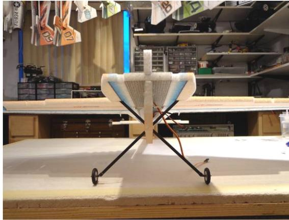
Temporarily flip over onto it's wheels, and adjust the struts so that the airframe sits level
