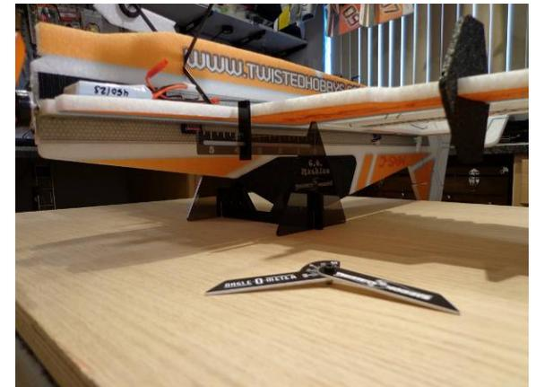
CG is 1.25" behind the spar or approx 3.56" from the leading edge of the wing.
