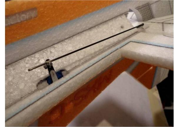
Install the Elevator Push Rod. Clip off any extra length.
