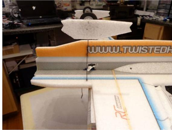
... as well as the bottom edge of the wheel pants being parallel to the bottom edge of the fuselage
