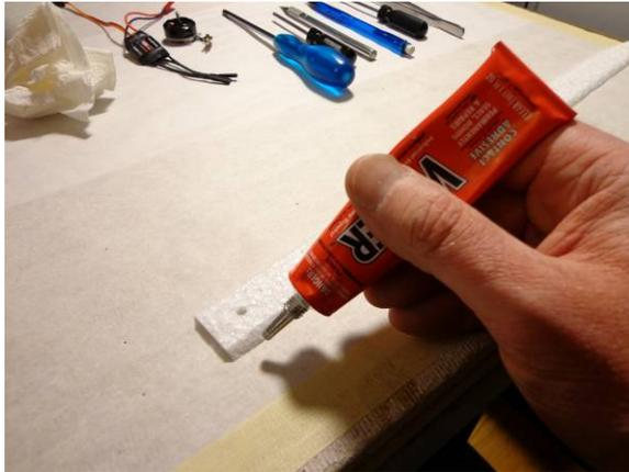
Install the trusses. Use tack up method. Apply glue to the truss, set in place, remove, let tack up, install. NOTE- leave one end free of glue as shown in next step. This can be cut off and used to re-enforce the motor mount or glued later
