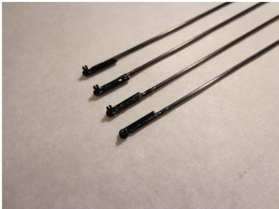
Carefully set pushrod in groove on snap-link, let dry for at least a few hours
