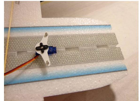
Install the aileron servo as shown. Note that the output shaft is to the REAR. Secure with a couple SMALL dabs of glue. Too much will make removal harder later if needed
