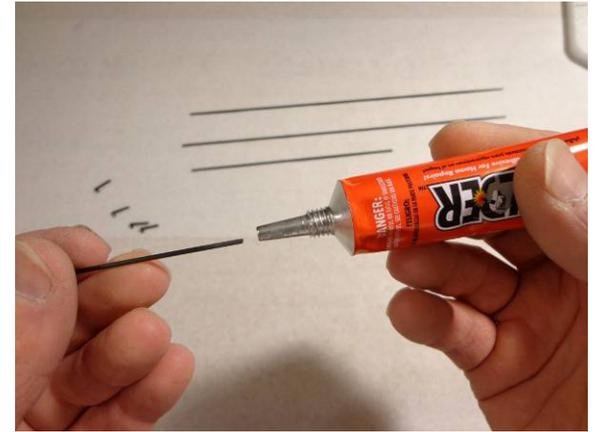
Put glue on pushrod by dipping it into the glue nozzle
