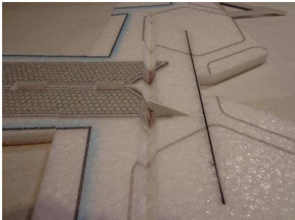
Glue elevator horn in. Make sure it is flush with the underside surface and that the hole is in line with the pivot point. Cut the slot deeper if needed
