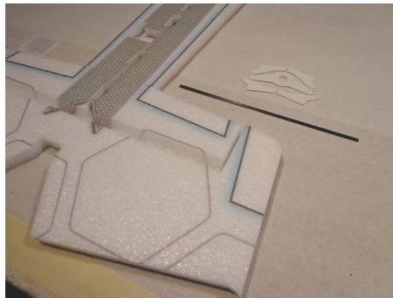
Locate the small rectangle carbon strip use to stiffen the elevator
