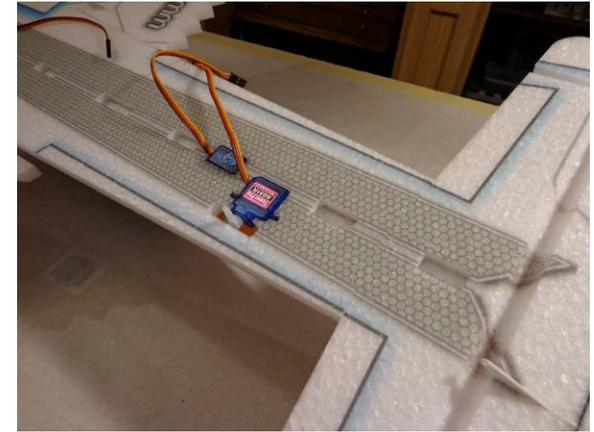
Install the rudder and elevator servos. NOTE - for extreme 3D control throws long servo arms are required. If not included in the servo hardware, fabricate by gluing on part of another horn. approx .75" is needed from center to link
