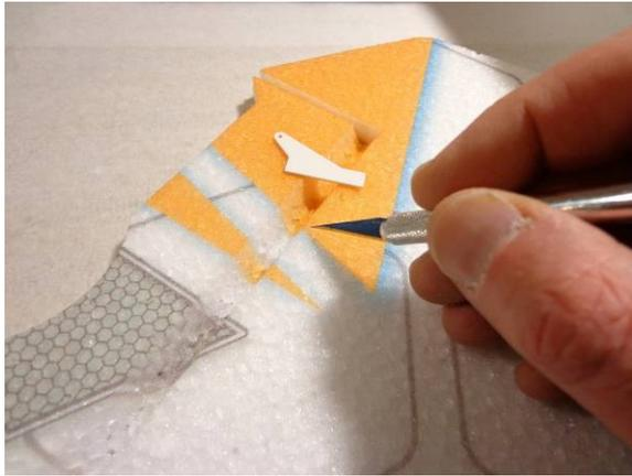
Install the Rudder Horn. Test fit in slot, cut out if necessary. Horn should be flush with the nearside surface
