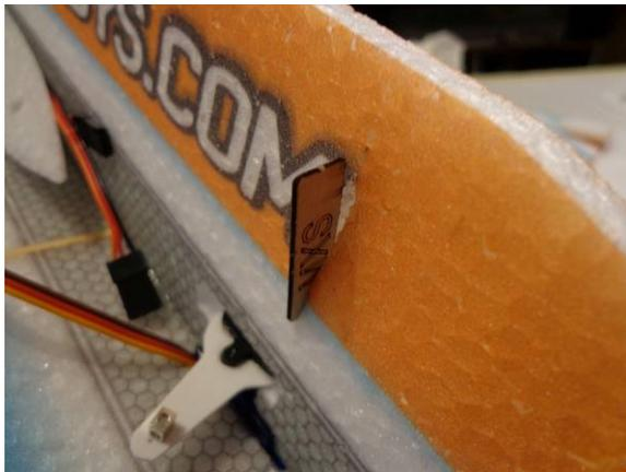
Slide the wood brace into the slot
