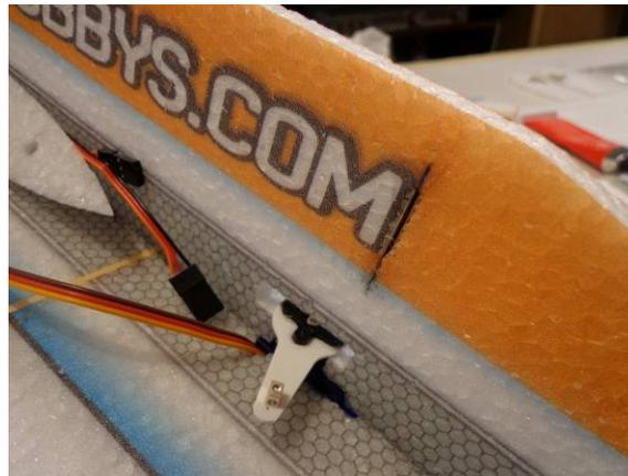
Center the wood brace within the thickness of the foam. NOTE- in the next step... one strut will insert on the back side, the other on the front side of the wood brace
