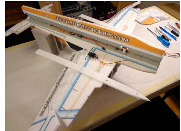
Install the trusses. Figure out first were you want to locate the RX and add servo extensions as required. NOTE- for rearward location only one extension on the ESC would be needed
