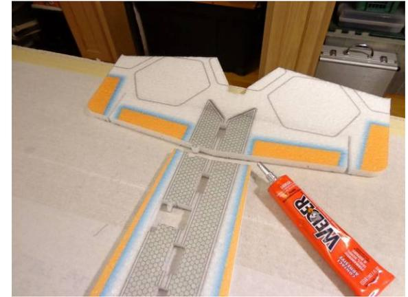
Locate the elevator/stab. Verify full down deflection is approx 50 degrees, carefully trim some foam from the bevel away if not. Apply glue via Tack Up Method
