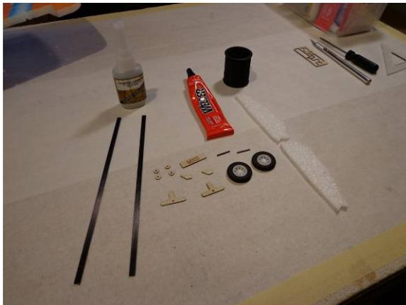
Prepare the Landing Gear. CA or Welders can be used. Wrapping with string will make it stronger. Remove all the tiny wood pieces from their plywood pack
