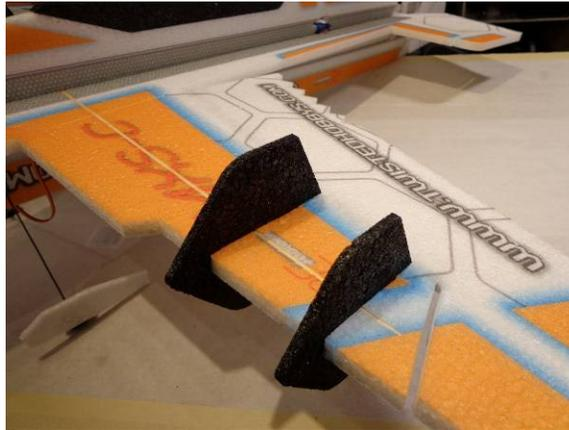
Attach the SFGs. Smaller ones outboard, and shorter side of both, down
