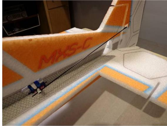
Install the Rudder Push Rod. Clip off the extra push rod length and save for the tail skid
