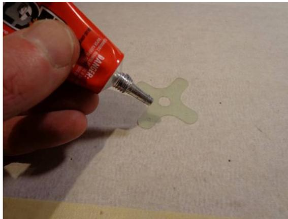
Apply glue to the mounts, install on nose, remove from nose, allow to tack up for approx. 5 minutes, assemble onto the airframe
