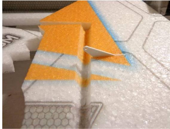
Glue the horn in. Flex the rudder back and forth to make sure the horn does not interfere. Hole in the horn should be in line with the hinge point
