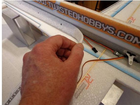
Carefully install the trusses. Make sure everything remains square. Leave one end free of glue until radio gear is installed. Handy for tucking the wires away
