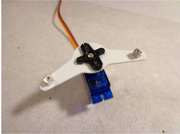
Complete the Aileron servo setup as shown. Make sure the servo is centered. Use inside holes for links. Servo horn and diff horn are glued together with Welders. NOTE - Output shaft is to the REAR of Airframe.
