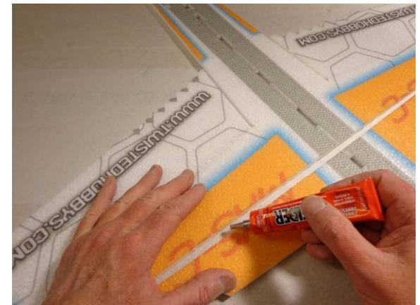
Lay parchment paper down on work surface. Spread glue inside the spar slot
