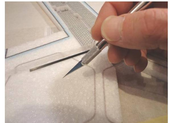
Locate the spar slot on the underside, cut deeper as needed. Test fit, spar should be flush with the underside of the elevator. Glue in, wipe away any extra glue
