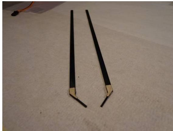
Glue the angle braces and axles to the struts as shown. NOTE- make a LEFT and RIGHT hand version. Wrap with thread, Soak with CA or coat with Welders
