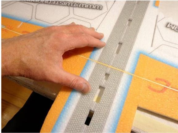
Insert spar, press fuselage/wing assembly together to ensure good glue joint on spar
