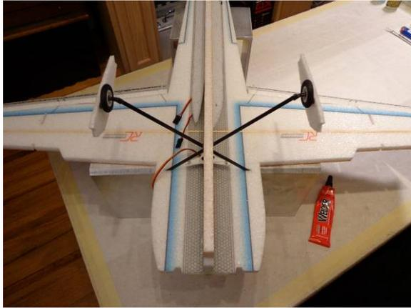
Make sure the wheel pants are parallel to the length of the fuselage
