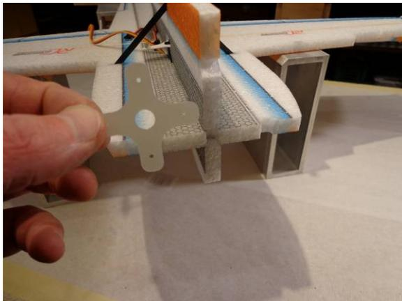
While the landing gear struts are drying, glue the fiberglass motor mount onto the front of the fuselage. Use the tack up method
