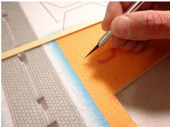
Cut out tabs that hold the wing and fuselage together so that the spar can be inserted
