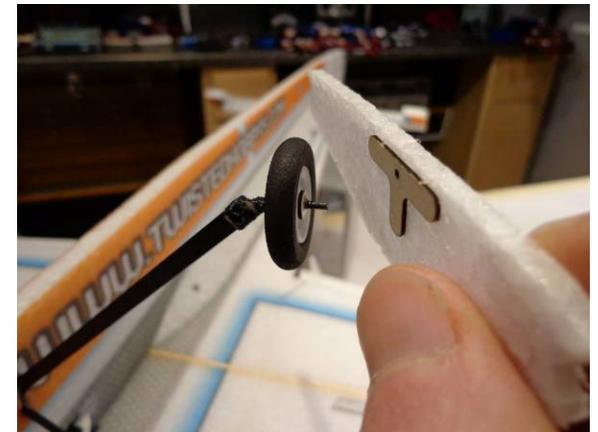
With the nozzle of the Welders tube, force some glue into the hole of the wood T-Brace, and apply a thin coat to the axle. Assemble the two pieces. Repeat for the other side
