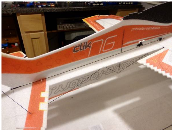
Dry fit the ends of the guides into the pre-cut holes. Use a small flashlight to help locate the holes.
