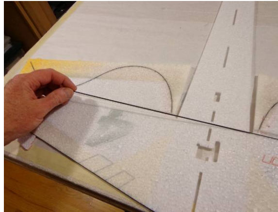
Lay the spar into the slot just forward of the aileron hinge bevel
