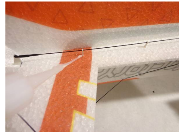
Once satisfied, put a drop of thin CA at the base of each guide and hit with Kicker
