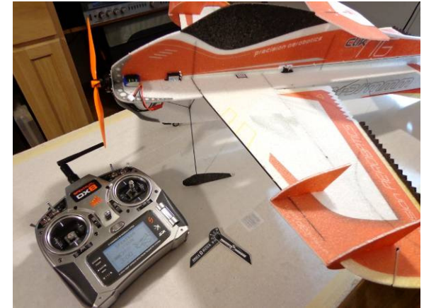
Program in approx 60% expo on the ailerons and 40% expo on the rudder and elevator
