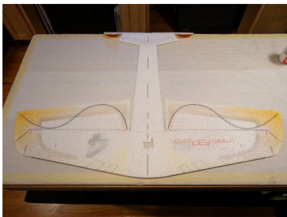
Leading edge strip installed, weights and pins taked away
