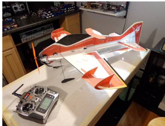
Locate the battery so that the CG is 245mm from the nose of the aircraft. Cut a hole or attach with Velcro if wanting to experiment with the CG point
