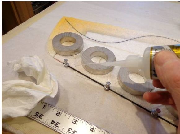
Apply CA to the edge of the strip so that it wicks in behind the strip
