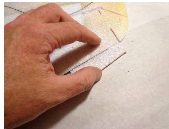
Assemble the two parts once the glue has tacked. Note that they are notched for the leading edge strip. Repeat for the other side
