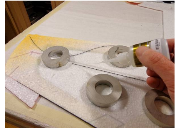
Apply thin CA and hit with Kicker
