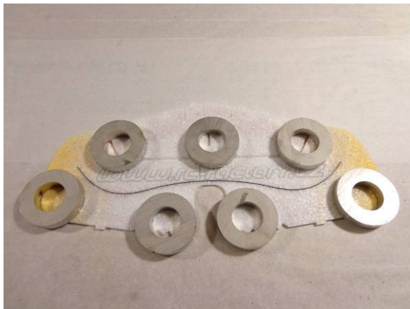
Before applying the CA, make sure everything is constrained in a flat position
