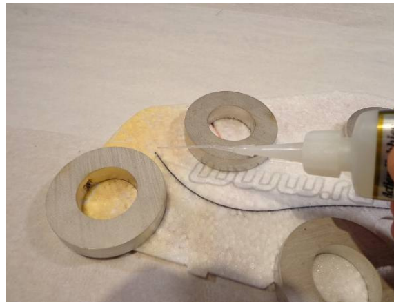
Apply thin CA and let it wick in around the strip
