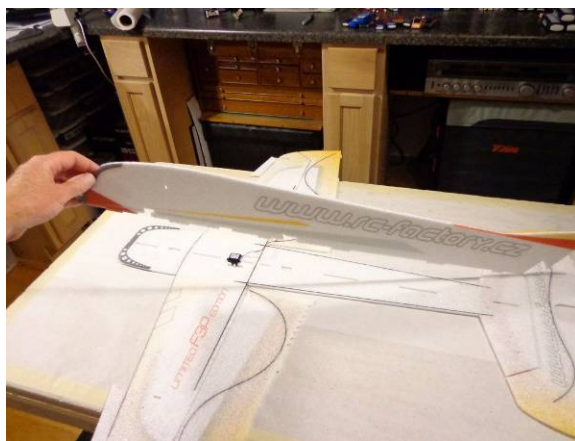
Test fit the lower fuselage section
