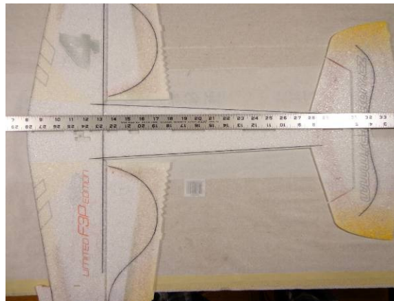
Cut them to length and fit into the precut slot. Make sure all the fuselage slots are still in line with each other. They will raise up slightly where passing over the wing spar
