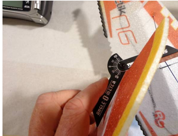
Adjust rudder control throws to +/- 45 degrees
