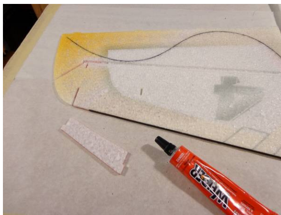
Use Welders and the tack up method to attach the leading edge extenders
