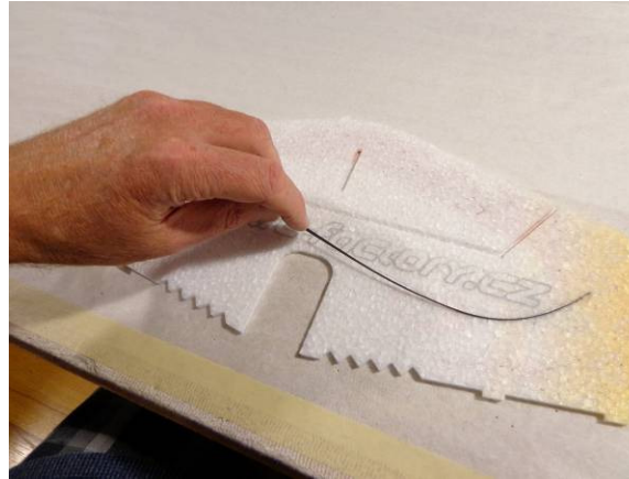
Test fit the strip into the precut curved slot, it should fill the slot from end to end
