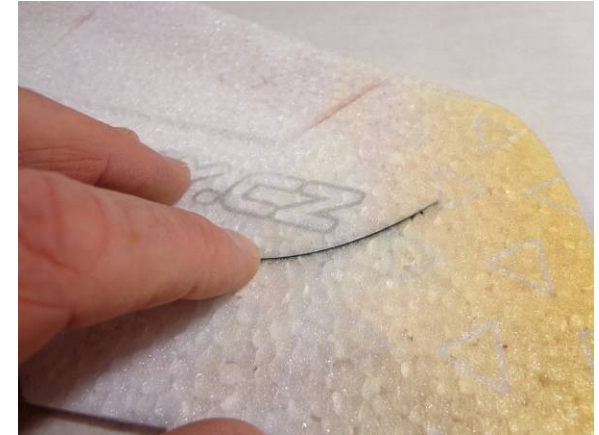
Make sure that the strip is flush to the surface of the elevator over the entire length
