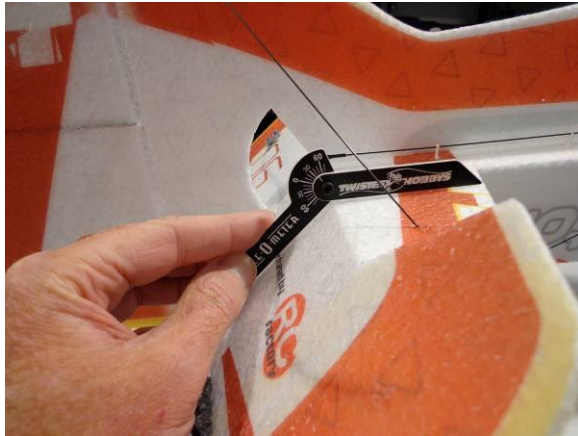
Adjust elevator control throws to +/- 45 degrees
