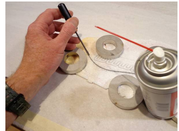
As you hit the area with Kicker, hold the strip down, sometimes it will rise out of the slot as the Kicker is curing the CA
