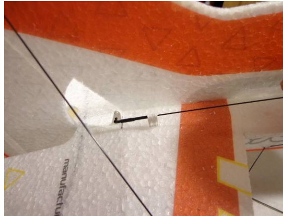
Position the snap link end of the push rod as shown....
