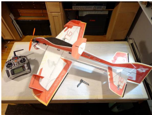
Control throws and expos can be adjusted to suit flying style and the size of the space being flown in
