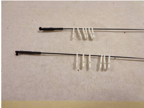
Slide 6 of each on to the two longer push rods as pictured above
