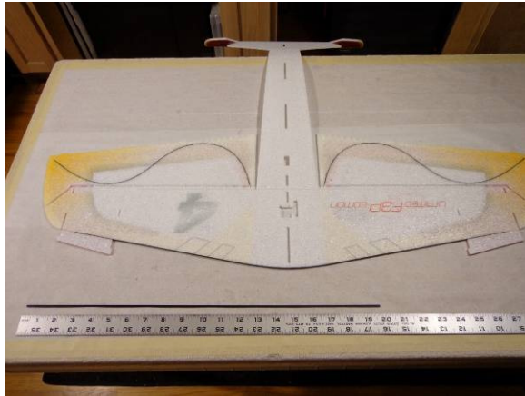
Locate the 3mm x 0.5mm x 500mm (approx 20in long) spar
