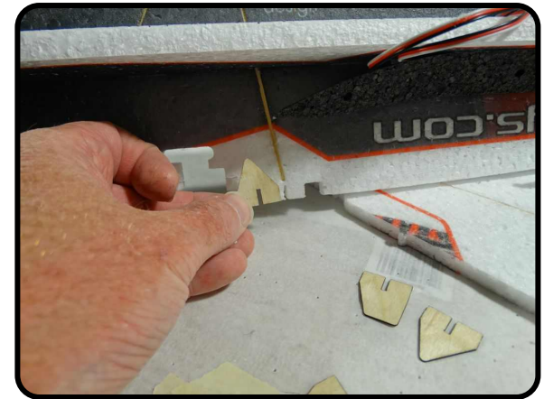
The pointed one is installed on the lower part of the fuselage.
