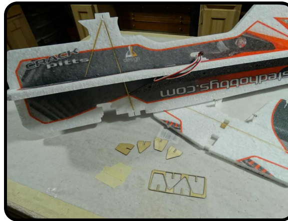
Locate the small wood fuselage doublers as pictured above. Note that there are two different kinds.
