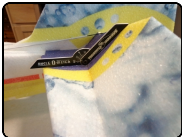
Elevator - set for approx \pm 45 degrees.
