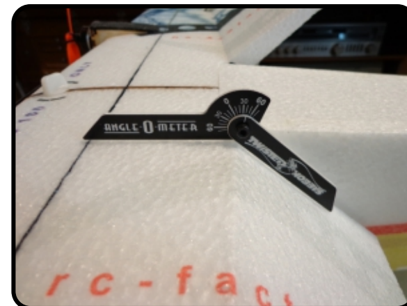
Now is also the time to set the control throws.... Aileron should be set to approx \pm 40 degrees
