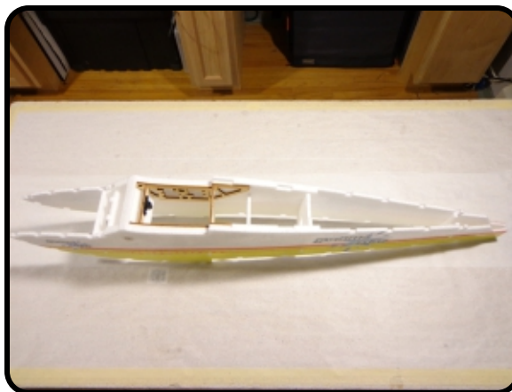
DRY FIT - looking down from the top, everything should be pretty square as assembled if all the tabs and slots have mated up properly.
