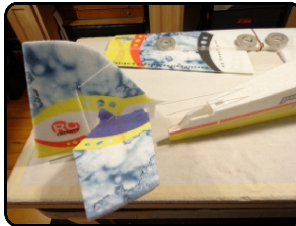
Once the tail section has dried, it can be attached to the main fuselage. Test fit everything first, so you know how it all goes together.
