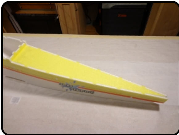
DRY FIT - the belly pieces into their location. If everything is assembled correctly up to this point there should be no trimming needed.
