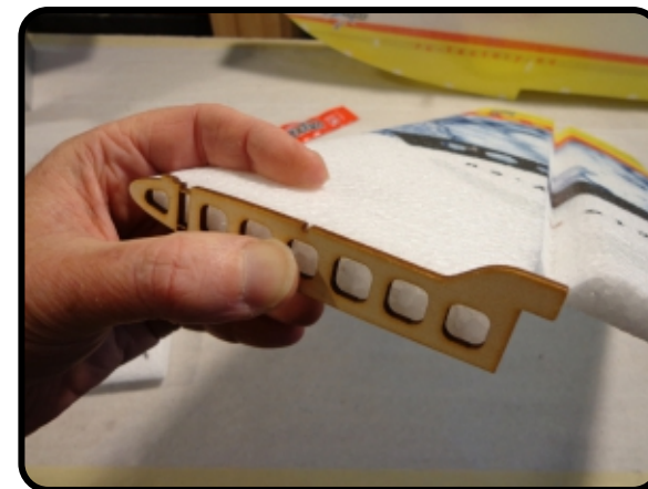
Once the glue has tacked up, attach the two pieces. If the profile or the rib does not match perfectly to the wing, use the REAR and BOTTOM edges as the ones to line up flush with.
