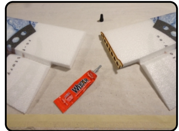
Using the tack up method again, coat the mating surfaces with a medium skim coat of Welders and allow to tack up.
