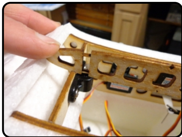
Note how the open area of the wing rib lines up with the center of the black plastic nut flange. Later, the included plastic thumb screw will pass thru this area and hold the wing in place.
