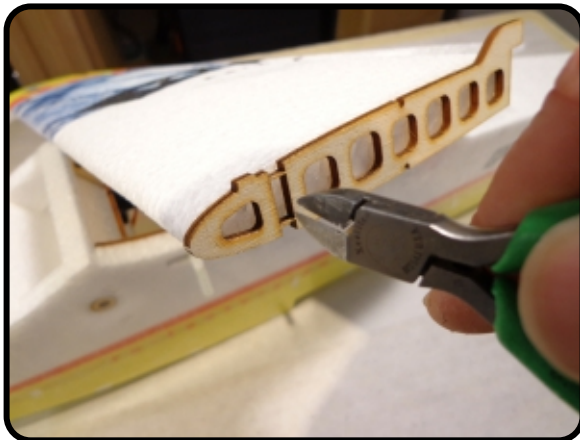
Snip away the little connector spacers.
