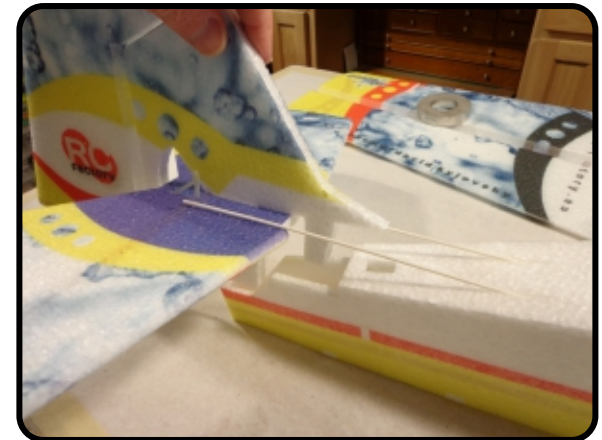
Make sure the push rods are on the TOP of the elevator.
