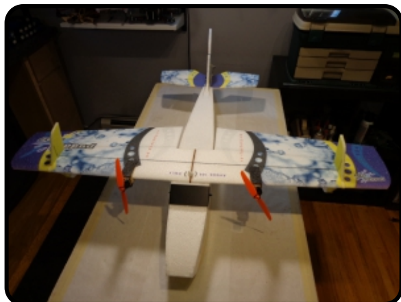
If using independent throttle channels for each of the motors, a mix can be setup to augment rudder control with differential thrust.
