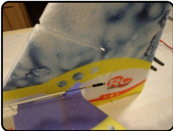
Deburr the end where cut and slide into the ferrule. Make sure that the rudder is still centered.
