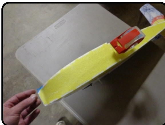
Grasshopper AND Waterbug Build - with Heavy Duty or clear Gorilla tape, cover the bottom surfaces. Trim flush and seal the edges with Welders
