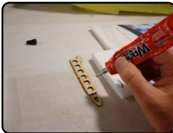
Use the Tack Up Method.... coat one side of the rib and the mating surface of the wing core with a medium skim coat and let sit for about 5 minutes.
