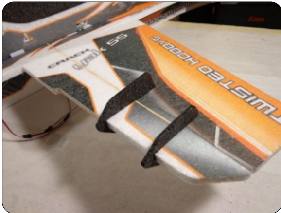
Install the SFG and repeat for the other three pieces
