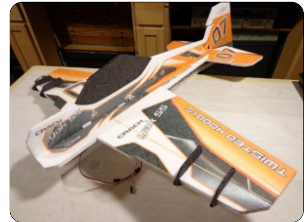
Next steps are optional, but will help to reinforce weak areas and increase durability. Four places around the nose/motor mount and ten places at the end of hinge lines and fuse stress
