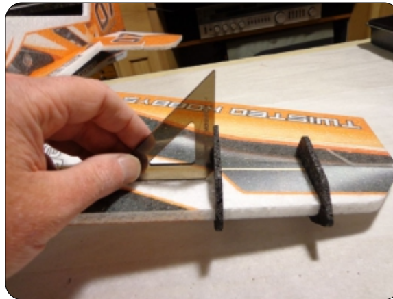
Before the glue dries, make sure the SFG's are square to the wing
