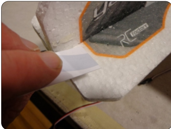
Spread it out to approx the area that the tape will be. Repeat this for all the areas in which Blendederm is being applied. Let the glue tack up for about 5 minutes
