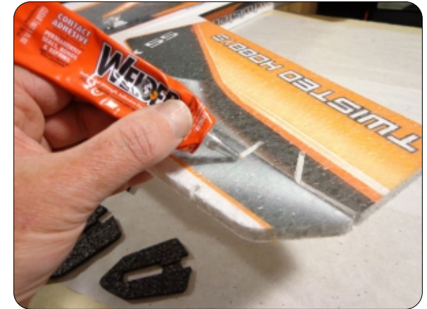
Apply a small bead of Welder's to the mating area on the wing
