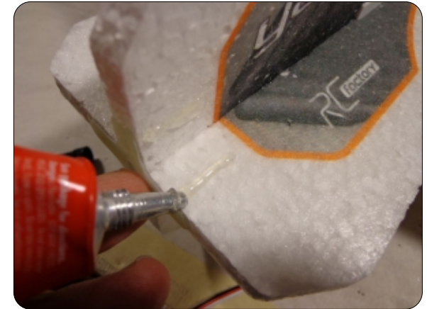
Starting with the motor mount area, apply a bead of Welder's approx as shown
