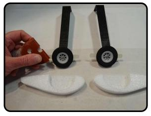
With some course sand paper, roughen up the areas where the foam pants and pant bracket will be joined together.
