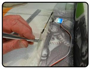
Make a slit for the horn. It should be deep enough so the corn at the back of the horn is flush with the foam and the front of the horn matches the profile of the hinged area.
