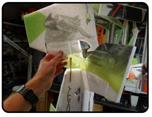
Once the wood pieces for the rudder are dry, the rudder can be installed. Apply some glue and join the two pieces.
