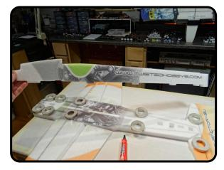
Once the previous step has dried, it is time to attach the lower horizontal fuselage piece. Test fit, then apply glue. Note - avoid glue in the areas noted in the next two pictures.
