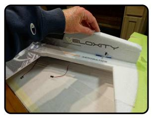
Join the two pieces together, make sure to feed the rudder servo wire thru the correct side like in the test fit.
