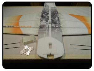
Once you are happy with the fitment and understand how all the part are installed, remove them all and prepare to re-assembly with glue
