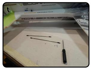
Get the tail control rods that were built in an earlier step and the remaining four little slotted head screws
