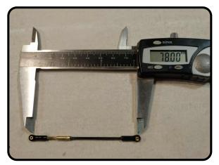
Install on of the other ball links onto the free end of the rod. The rod may need to be sanded a little. 78mm from hole to hole is the goal. Attach with CA and Kick.
