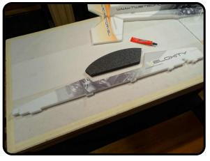
While the previous step is drying, attach the canopy to the upper vertical fuselage section. Tack up Method can be used for this step.
