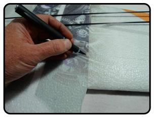
Make sure the slit is clear where the wing and fuselage meet. Test fit the spar to make sure it sits flush to the surface of the wing.
