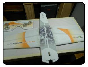
.... to the work surface in the area of the slit for the spar. This will ensure that the leading and trailing edges will locate at the center of the fuselage. Repeat for the other wing.
