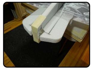
Put some tape around the nose so that the front tabbed pieces are pull back towards the motor mount a little. Don't over do it... just enough so all the surface are firm against each other.
