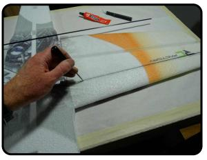
Install the spar, make sure that it is fully seated and flush to a little below the surface of the wing
