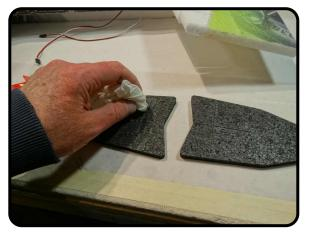
Install the carbon rectangles back into their slots, make sure they are flush and wipe away any extra glue. Set aside on a flat surface to dry.
