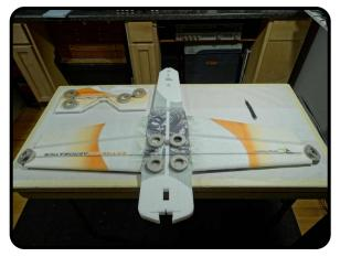
Flip back over so that the under side is facing up. Weigh down with some heavy objects as shown and let this thoroughly dry before handling again.
