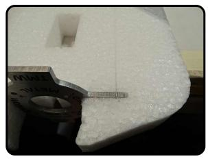
Slide the mount into position, working it a little from side to side to get good glue distribution. Make sure the slots and motor mount notch line up.
