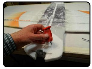
Flip the airframe over now so the BOTTOM SIDE is facing up. Squeeze some Welders into both to the slits.
