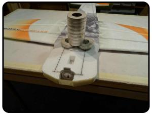
Apply some weights to the whole thing and let it set like this until the glue has dried. Note a piece of tape is being used to keep the front tabs of the nose in contact with the motor mount.
