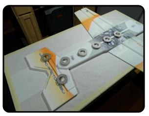
Make sure the two pieces are fully seated to each other. If so, squareness should be really close, double check with a tape measure by measuring from elevator tips to the wing tips.
