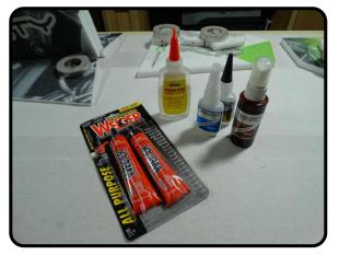
Welders, Foam-Tac or CA can be used as the primary method of joining the parts. This Build will use Welders for all joints unless called out otherwise. Two to three tubes of Welders are needed.
