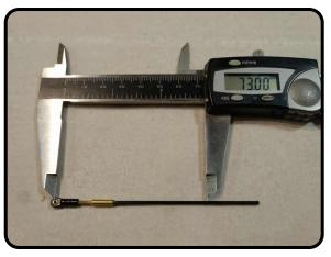
From the CENTER of the hole of the bass ball in the ball link, measure off 73mm and cut the rod. Use a rolling action with a hobby knife to score the rod, then snap apart at that position.
