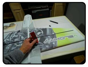
Flip the assmebly over and repeat for the top side spar. Fill the slit with glue, and install the 1000mm long spar.
