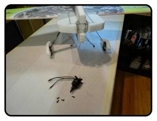
Locate the motor you will be using and its mounting hardware. For the Upgrade mount, four 3mm allen head cap screws, for the wood mount, the four longer self tapping screws
