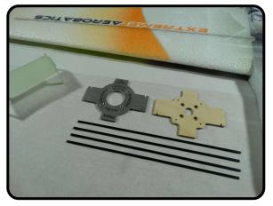
Firewall and associated carbon stiffener spars are next. Locate the motor mount and four 2.5x1.5x200 carbon rectangles. Note the metal mount to the left is an Optional Upgrade part.
