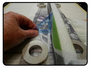
Once it is all pressed together, wipe away any extra glue and check for squareness along the length of the fuselage. With the thickness of the foam it should be pretty square on it's own.
