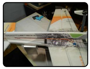
With the Twisted Hobbys Power Combo, the servos have extra long leads, so extensions are not needed. Note the location of the Crack Receiver.
