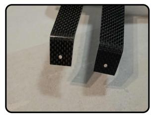
Drill .112" (3mm) dia holes in the landing gear as shown. Note the location is not super critical, just locate approx as shown and make them similar to each other
