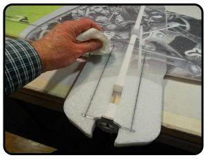
Install the TOP SIDE rectangles by squeezing glue into the slit and pressing them in, make sure they engage the motor mount and wipe away any excess glue.
