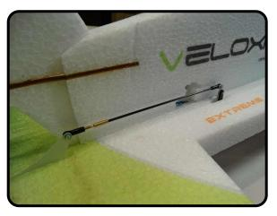
Install the elevator control rod as shown. Note that the ball links have a flat flanged side, this is the side that mates with the horns. Apply a little thread locker and install the screws.
