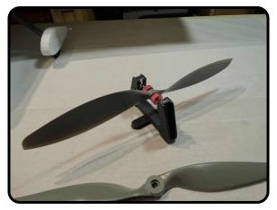
Balance the props you will be using. With the 100g TMW motor, a s12x6e prop can be used.
