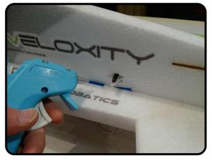
Now is a good time to apply a bead of low temp hot glue to any places where the servos meet the foam.
