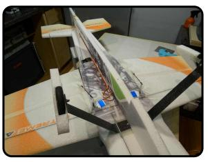
Under side showing one way to locate the electronics.
