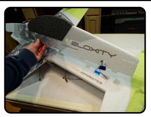
Test fit the top fuselage section. Make sure and feed the rudder servo lead thru to the same side as was done with the elevator servo lead.
