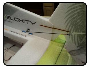
Repeat the process for the rudder control rod. With the servos centered, fine adjustment can be made from the threaded end ball link to get the control surfaces perfectly positioned.
