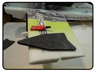
SFG's will be joined to the end of the wings with the Tack Up Method. Apply a skim coat of Welders to both mating surfaces. Note that the carbon slits face inward.
