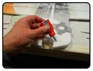
Start by attaching the motor mount. Put some glue into both the left and right slots as shown.
