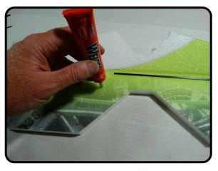
Start from the top side and with the 3x1x250 spar. With the tip of the Welders' nozzle, squeeze glue into the pre-cut slot.
