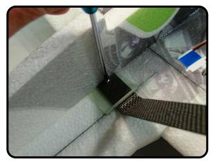
Back the screw out about 2 or 3 three turns so that it clears the thickness of the LG strut. Install the strut and tighten the screw.
