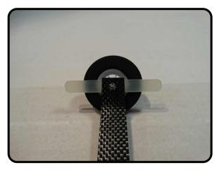
Adjust the hex nut on the inside of the wheel hub so there is minimal clearance and the wheel can still spin. Use a dab of Welders to lock it position. then finish assembling the items
