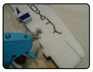
Put a little hot glue on the edges of the cut out.
