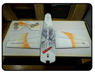
Wings are joined together next. Note that the bottom of the fuselage (side with the servo cut outs) and the bottom of the wings should be facing UP.
