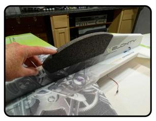
Firmly press up and down the length of the upper fuselage piece to ensure the two pieces are fully seated to each other. Do this a couple times.
