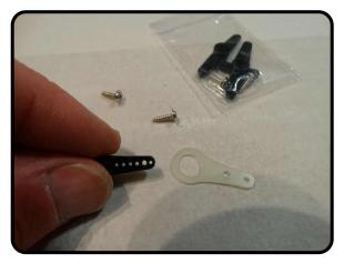
Enlarge the second in servo horn hole to .060" diameter and match drill a .080" dia hole in the fiberglass servo extension arm. Repeat this for all four arms. Get 4 screws from the servo bags.
