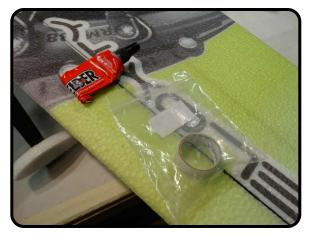
Add a 1.5" length of Blenderm to the extreme ends of all the hinge lines. Apply a thin patch of Welders under where the Blenderm will go. Doing this will strengthen the hinges
