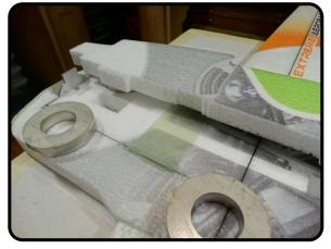
Avoid glue in the area where the carbon landing gear struts will pass.
