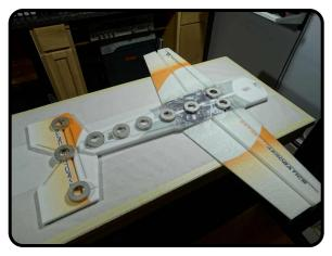
Let this dry a little while before handling. Weigh everything down to ensure that the assembly dries in a nice and flat condition.
