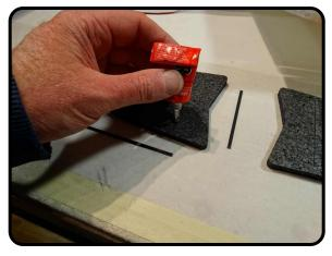
After verifying fit, remove the carbon rectangles and squeeze a little Welders into the slots.
