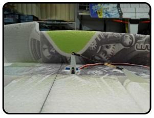
Once you are happy with everything, install the servo with a medium dab of low temp hot glue at the bottom of the pocket, and the horn with Welders into the slit that was cut.
