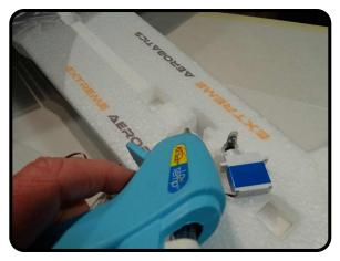
Apply a little low temp hot glue to the sides of the hole and install the servo. Servo lead should stick thru underneath, install the servo quicky, the hot glue sets fast.
