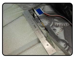
Press the servo back into is pocket, and with a straight edge, align the base of the control horn with the angle of the servo.
