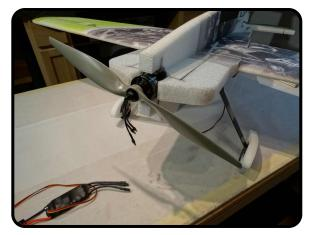
Install the motor with the wires off to the side in which the ESC will be mounted.
