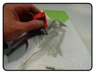
Squeeze some Welders into the control horn slot and apply a skim coat of Welders to the base of the horn.
