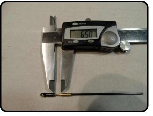
Thread the ball link onto the ferrule until there is approx 6.5mm between the shoulder of the ferrule and the open end of the ball link.
