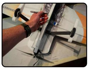
Make a part on the fuselage 275mm back from the nose for the CG point.
