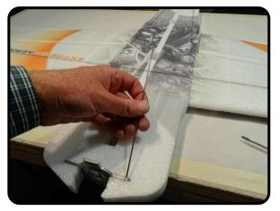
Install the rectangles like was done on the top, and again making sure that they engage the notches in the motor mount
