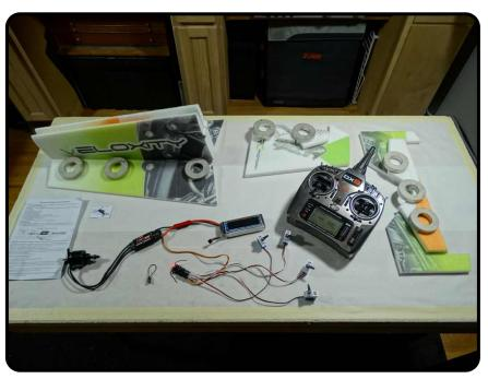
Start the build by locating the two wings, the elevator and the rudder. Fold back as shown and weigh them down for about an hour to loosen up the hinge area. Now is also a great time to setup your radio and to test that all your electronics are functioning properly.
