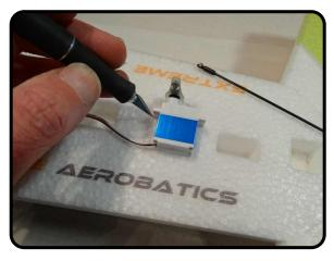
Cut slits for the servo tabs like what was done with the aileron servos, and test fit to make sure it will sit flush with the near surface.
