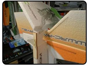
Make sure the rudder aligns with the wood pieces and that it is straight and true with the main part of the fuselage.
