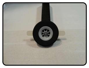
Once all the items are attached, check that the wheel still spins freely and that the pant bracket is perpendicular to the landing gear strut. Repeat the previous steps for the other strut.
