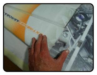
Make sure that during the "transfering" of glue process that an even coat is on both mating surfaces. Let set for about 5 minutes. Then join the pieces making sure to apply pressure....
